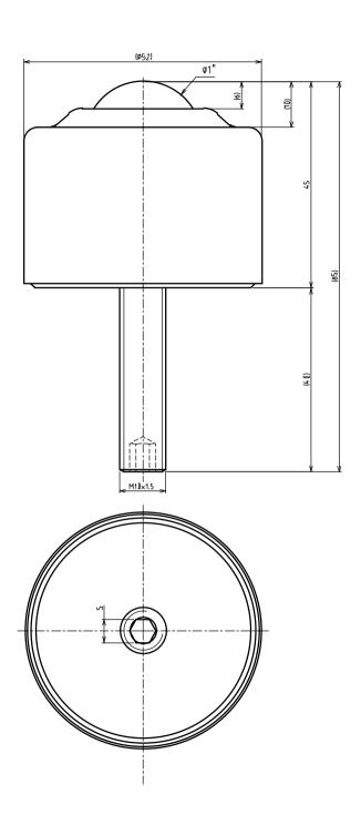
>Description IS-N Type Ball Transfer With Sturdy Bolt IS-25N Type Unit = mm
