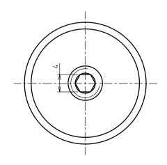
>Description IS-SN Type Ball Transfer With Sturdy Bolt IS-13SN Type Unit = mm
