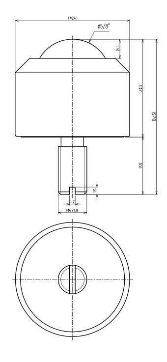
>Description IS-SN Type Ball Transfer With Sturdy Bolt IS-16SN Type Unit = mm
