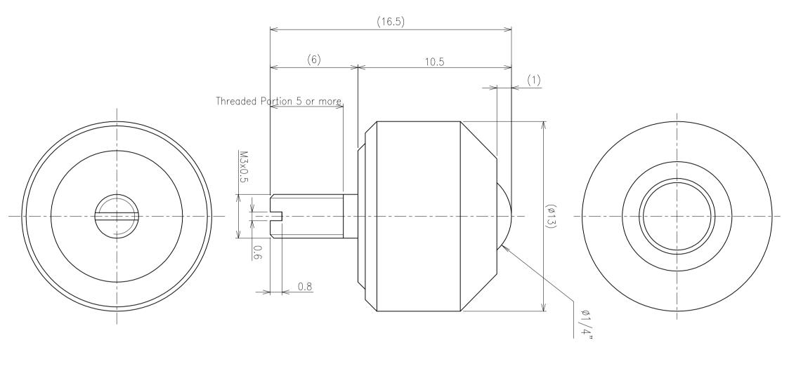
>Description IS—SNM Type Ball Transfer With Sturdy Bolt IS—06SNM Type Unit = mm
