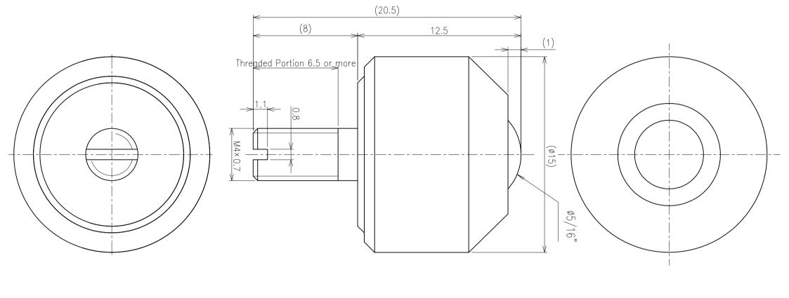
>Description IS—SNM Type Ball Transfer With Sturdy Bolt IS—08SNM Type Unit = mm
