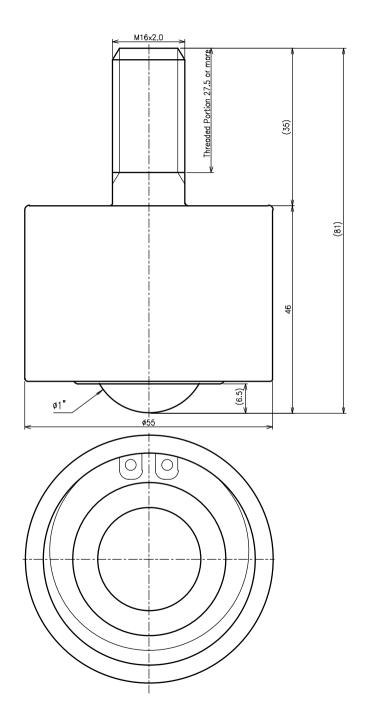
>Description IK—N Type Ball Transfer With Sturdy Bolt IK—25N Type Unit = mm
