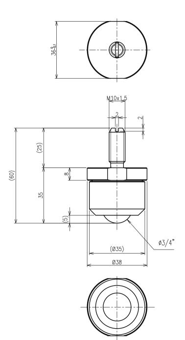
>Description IK—SNM Type Ball Transfer With Sturdy Bolt IK—19SNM Type Unit = mm
