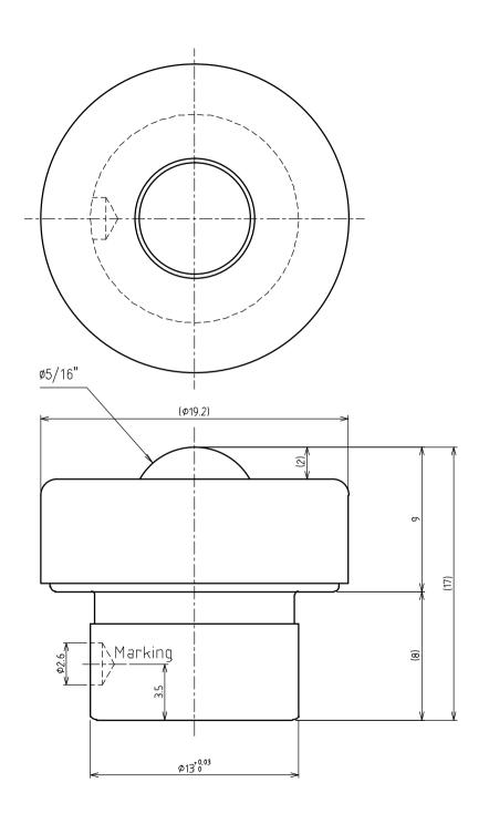
>Description S Type Stroke Ball Transfer S-08 Type Unit = mm
