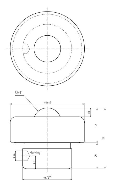
>Description S Type Stroke Ball Transfer S-10 Type Unit = mm
