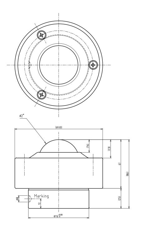
>Description S Type Stroke Ball Transfer S-51 Type Unit = mm
