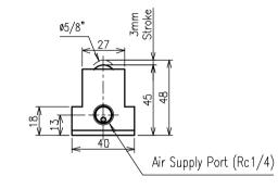
>Description ISR—T Type Air Ball Lifter ISR—28T—400 Type Unit = mm
