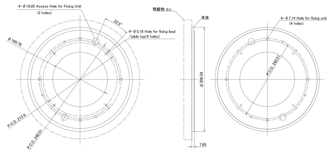
Note 1: Please place this unit on a flat surface, during usage. This unit is not meant for sideways use or suspended use. Please note that the load limit is in reference to the the whole load on the unit, which also includes the table top. The load limit does not include impact force. Moving the load by sliding it on the table top, or forcefully shaking the load may cause the unit to malfunction.
