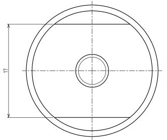
>Description IS-N Type Ball Transfer With Sturdy Bolt IS-16N Type Unit = mm
